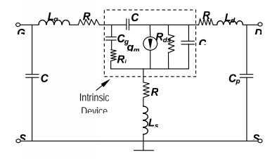
Figure 3: AMCAD small signal Model for HEMT
