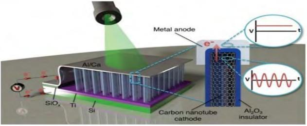
Optical rectenna schematic. This schematic shows the components of the optical rectenna developed at the Georgia Institute of Technology.
